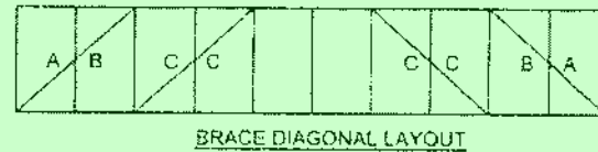
BRACE DIAGONAL LAYOUT
