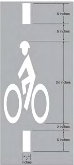
Figure 9C-7. Bicycle Detector Pavement Marking
