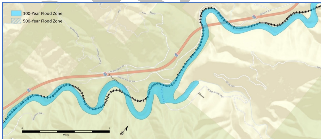
Figure 71. Flooding exposure of the Union Pacific Railroad in the Sacramento River Canyon, near Pollard
